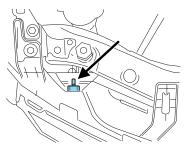
7. HORIZONTAL AIM IS NOT REQUIRED FOR THIS VEHICLE AND IS NON-ADJUSTABLE.
